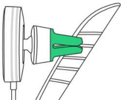
Slide the prongs of the Velox onto your vehicle's air vent blades.
